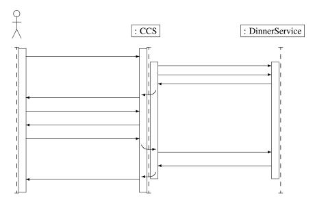
Figure 13: Two services running in parallel (the curved arrows indicate where information needs to be transmitted between sessions)
