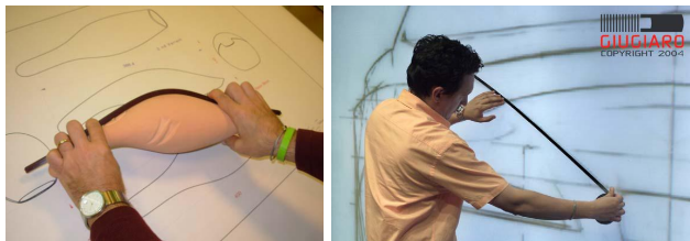
Fig. 2 Shape analysis and modification expressed using curves in industrial product design: left) a vacuum cleaner mockup and right) a car being reviewed
