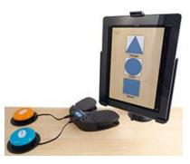
Figure 2 - Blue2 Bluetooth Switch by AbleNet®
