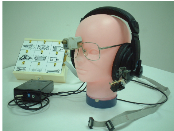
Figure 2.11: Infra-red home appliance control system
