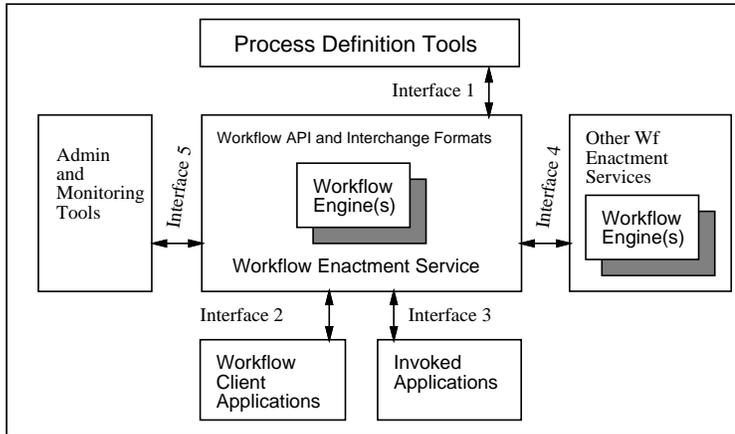
Fig. 4.1. WfMC Reference Model
