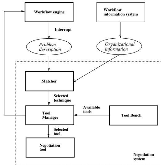
**Fig. 6.2.** An architecture for the Integration of workflow systems and GDSS tools
