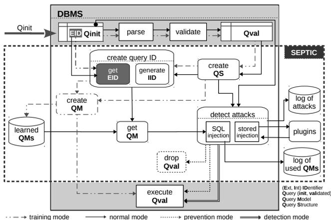
Fig. 2: Architecture and data flows of SEPTIC.
