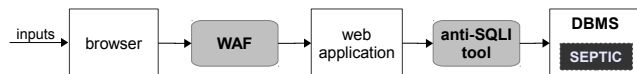
Figure 5: Placement of the protections considered in the experimental evaluation: SEPTIC, anti-SQLI tools, and WAF.
