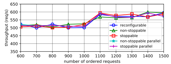
Figure 3: Throughput during an adaptation in a LAN.
