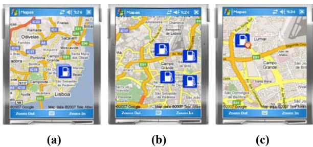
Figure 1 – Visualization of points of interest with: (a) aggregation symbol (b) individual symbols after zooming in (c) symbols with higher level of detail
