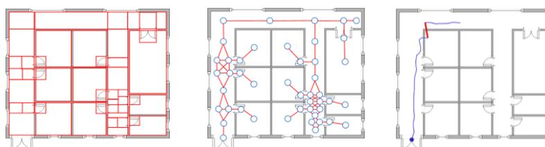
**Fig. 1.** Definition of the floor plan graph.
