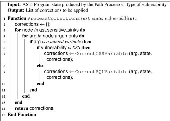
Algorithm 4: Algorithm applied by our Correction Processor.
