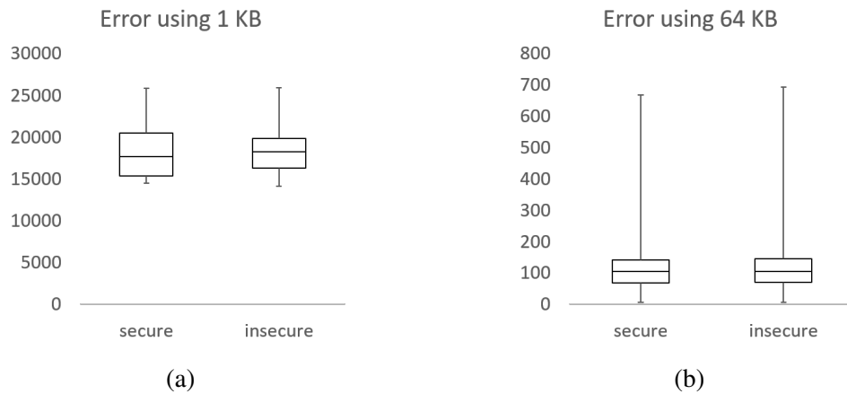
Figure 5.7: Errors in estimations returned by the secure and the original versions of Count-Min when monitoring by flow. (a) using 1 KB of memory (b) using 64 KB of memory
