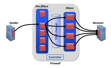
Fig. 2. Overview of the architecture and communication pattern with the firewall.
