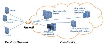
Fig. 1. Overview of a SIEM architecture, showing some of the core facility subsystems.
