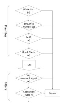
Fig. 3. Filtering stages at the firewall.
