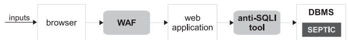
Fig. 7. Placement of the protections considered in the experimental evaluation: SEPTIC, anti-SQLI tools, and WAF.
