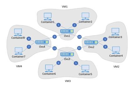
Figure 3.4: Example of substrate network
