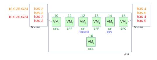
Figure 4.6: Chaining flows to different security functions
