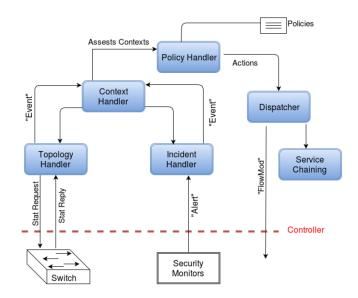
Figure 4.1: Security monitoring component: high-level architecture
