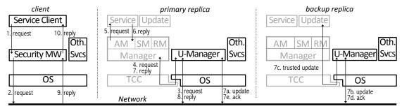
Fig. 1: Architecture of the Verified Passive Replication scheme. Light shaded parts correspond to the trusted system components.
