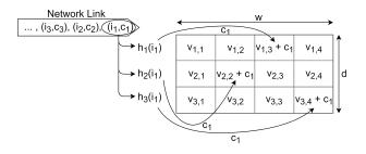
Fig. 1. Count-Min update operation. Data structure width w=4; depth d=3.
