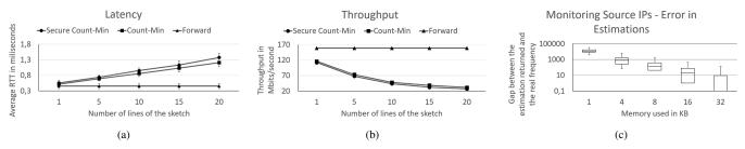
Fig. 3. (a) Latency between the two hosts; (b) Maximum throughput; (c) Estimation errors when monitoring by source IP address
