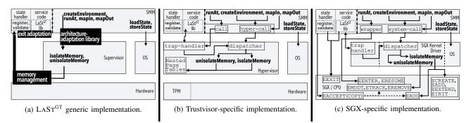
Fig. 4: LAST<sup>GT</sup> abstraction of non-common mechanisms (4a, black boxes). TC-architecture-specific implementations (4b and 4c).
