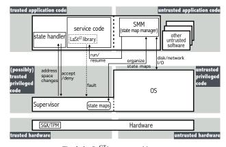
Fig. 3: LAST<sup>GT</sup>'s system architecture.
