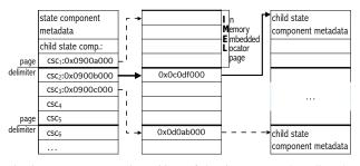
Fig. 8: IMEL pages contain positions of data in memory. They allow the LAST<sup>GT</sup> library to access a child state component (e.g., a chunk,  $csc_2$ ), and they help the untrusted code to locate such component and load it. Other IMELs (e.g., at  $csc_1, csc_3$ ) that are not accessed are not loaded.
