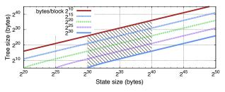
Fig. 6: Hash tree size (y) as a function of the state size (x) for different block sizes, with a 32 bytes hash (e.g., SHA256). Shaded area is our target.
