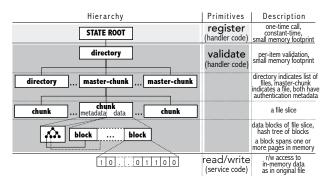
Fig. 5: State hierarchy. A directory can contain several master chunks and (sub-)directories. The relevant primitives (register, validate) build a chain of trust between the service reads/writes and the state root verified by a client.
