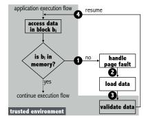
Fig. 1: Example of a program execution inside a trusted environment that offloads data I/O from storage or network devices to untrusted code.
