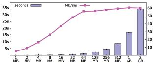
Fig. 12: Time (bars, left y-axis) and speed (line, right y-axis) to build the  $LAST^{GT}$ -compatible state for different state sizes.
