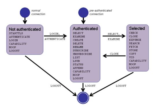
Figure 4: IMAP protocol finite state machine.
