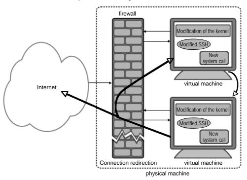
Figure 9- Overview of the high-interaction honeypot architecture
