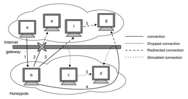
Figure 10- Connection redirection principles: example
