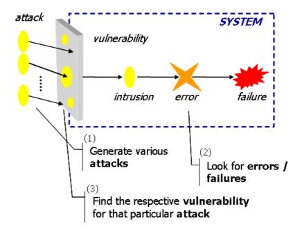
Figure 2: Composite fault model (attack, vulnerability, and intrusion).
