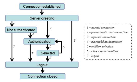
Figure 7: IMAP state and flow diagram
