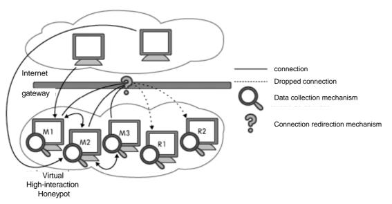
Figure 12- Overview of the most recently deployed version of the honeypot
