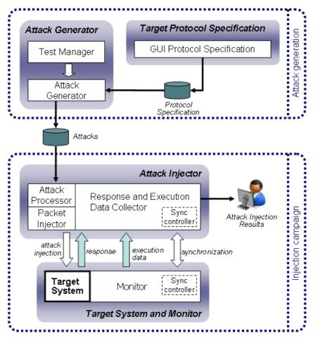
Figure 3: The architecture of the AJECT tool.
