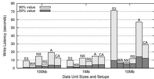
**Figure 5.** 50<sup>th</sup>/90<sup>th</sup>-percentile latency (in seconds) for 100kb, 1Mb and 10Mb DU write operation for a PlanetLab client at the UK. The bar names are the same as in Figure 4. DEPSKY-A and DEPSKY-CA are configured with  $n = 4$  and  $f = 1$ .
